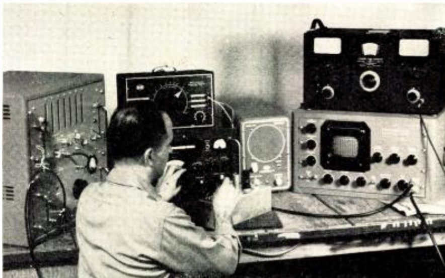
Fig. 3. Test position used to align sideband generator units. Equipment visible in photo includes a decade frequency meter, audio oscillator, receiver and SSB receiving adapter, and panoramic spectrum analyzer with a signal generator.
