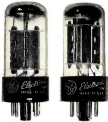
Fig. 1. One of these tubes is an old one that has been rebranded, the other is new. Note the thinner lines of the lettering of the tube on the right; it is the phony.
