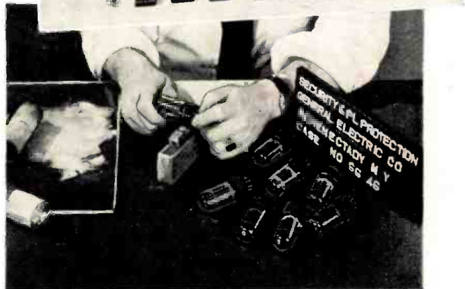
Fig. 5. How the counterfeit brand was put on a cleaned-up defective tube is shown.
