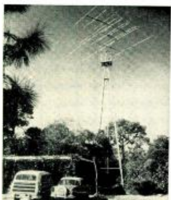
COVER PHOTO: Part of the “dream” antenna setup of W4YI and W4TFP, Sarasota, Florida. The Steinmetz “team” have their three Telrex beams mounted atop 50-foot mast. For details see article, page 38. (Ektachrome by Joseph Steinmetz)
